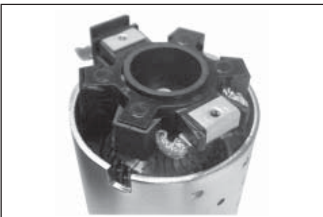
Figure 8-67. Installing Brush Holder Assembly with Supplied Tube.
